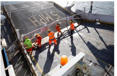
This week work was carried out to replace the main chains on the ferry which needs to be done ahead of the refit. Ferry chains need to be replaced every three years
